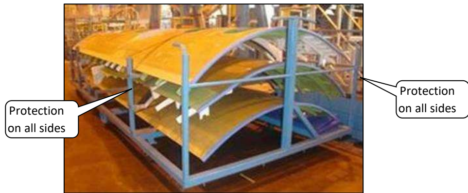
Figure 33: Example of transportation cradle, showing product with protection on all sides
