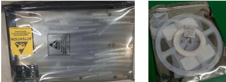
Figure 46-B: Example of shielded antistatic package (ESD)
