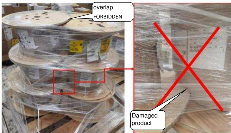
Figure 45-E: Coil on pallet – INCORRECT WAY - FORBIDDEN
