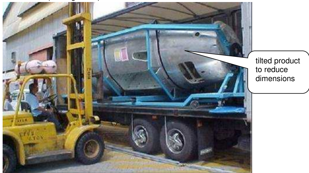
Figure 32: Example of packaging with tilted product, in order to reduce dimensions.
