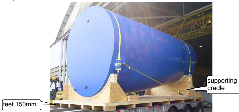
Figure 18: Example of base for large packaging, with cradle for material.
