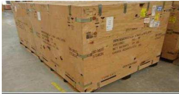
Figure 57: Example of closure with fast clips
