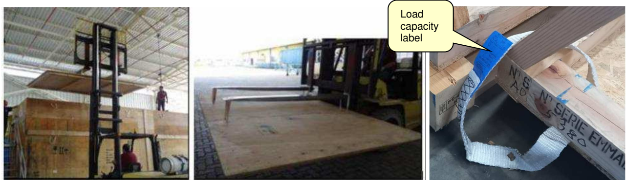
Figure 25: Example of handles to facilitate handling of lid parts. Handles with capacity label
