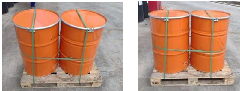
Figure 46-B: Example of drum with volatile products, without stretch
