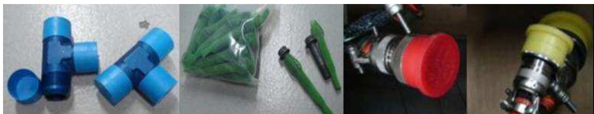
Figure 51: Example of items with individual protection
