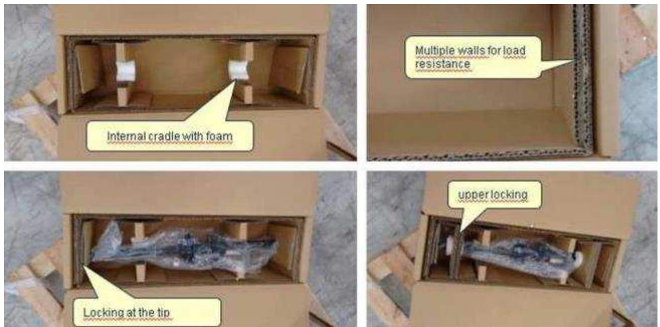
Figure 07: Example of cardboard packaging walls and internal cradle
