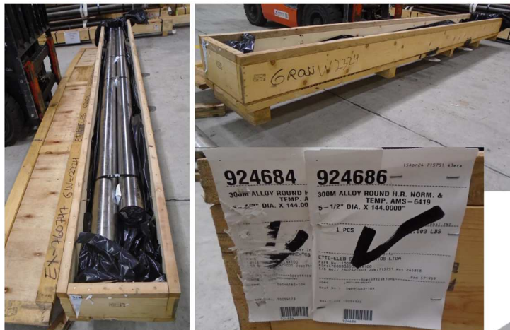
Figure 39-G: Example of round bar in reinforced wood box
