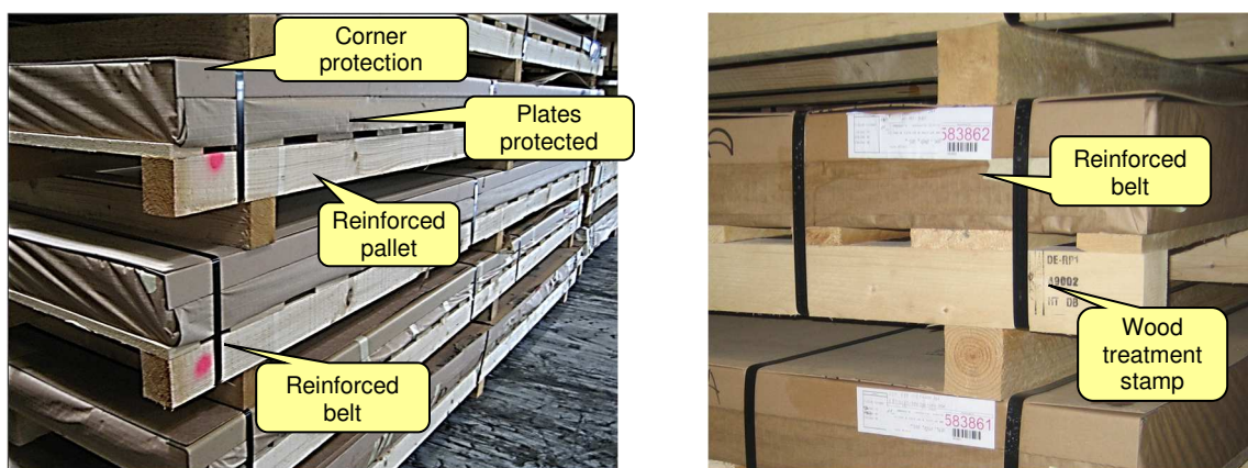
Figure 39-B: Example of palletized material fixed using strapping
