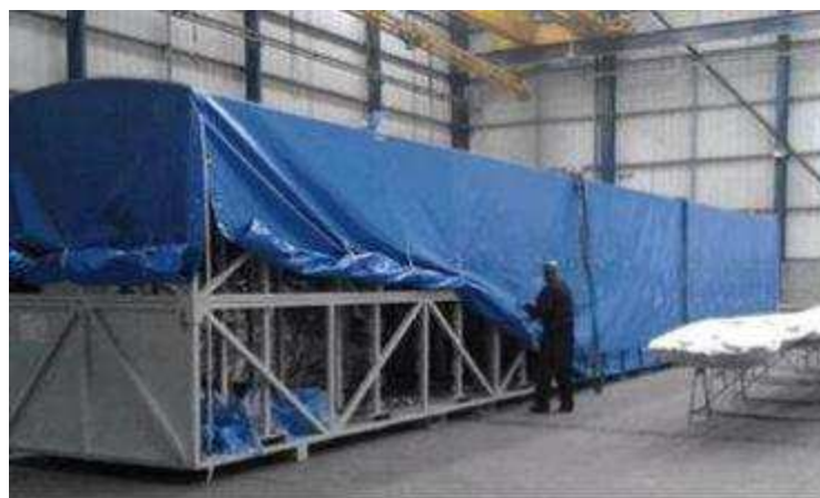
Figure 35: Example of returnable covering for container
