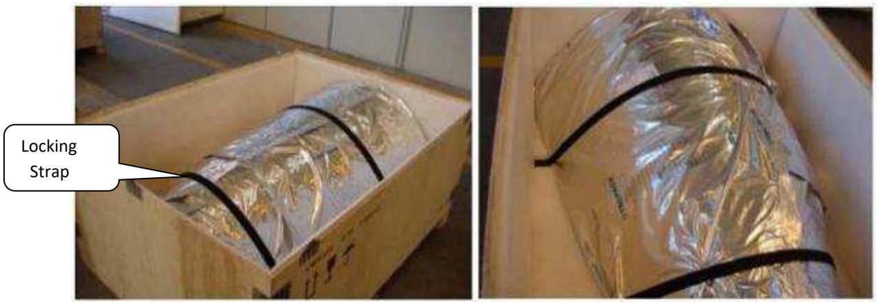
Figure 20: Example of securing large packaging done with straps
