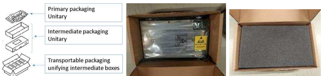
Figure 48: Example of packing for serialized or fragile items, or that are sent individually to production.
