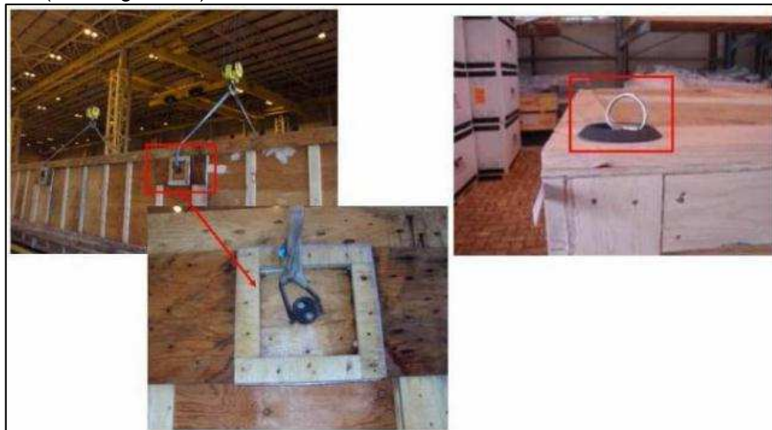
Figure 23: Examples of ringlets for bell type packaging.
