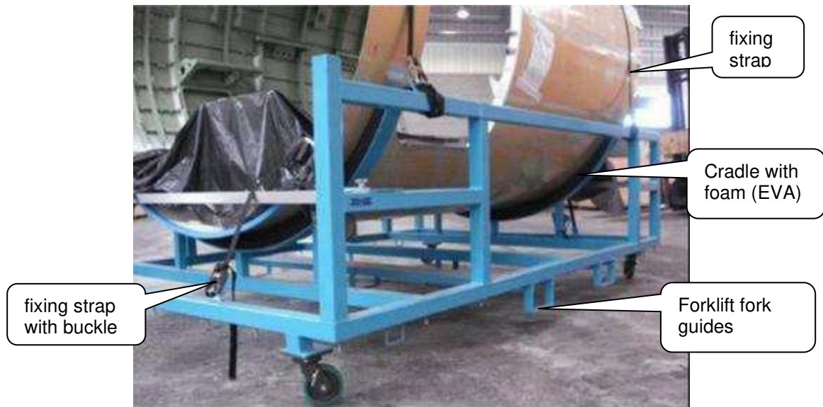
Figure 31: Example of product in transportation cradle, showing attachment strap with ratchet, attachment strap, support cradle with EVA, and forklift fork guides
