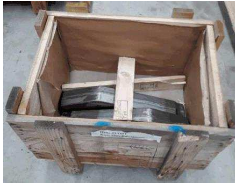
Figure 44-A: Example of internal locking of forged items
