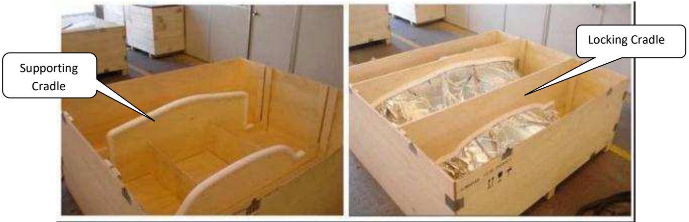
Figure 19: Example of securing large packaging made with plywood cribs
