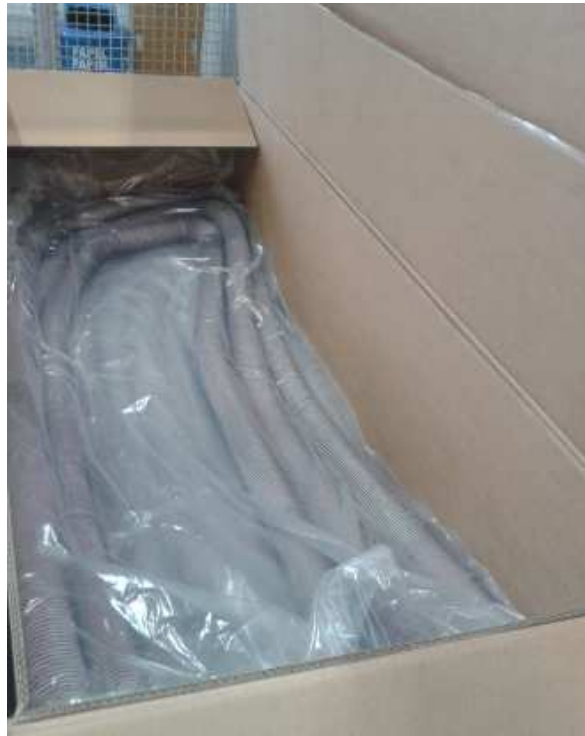
Figure 74: Example of ducts bent inside the box
