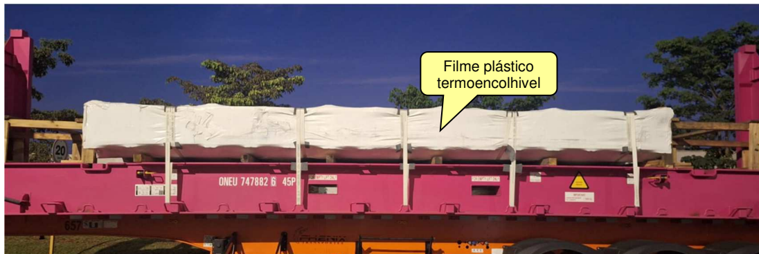
Figure 39-E: Example de protection over pallet on flat rack container (protective white shrink film)
