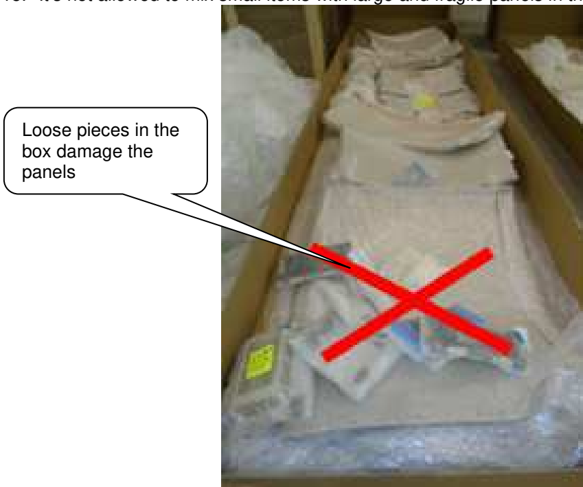
Figure 58-A: Example of box mixing Panels and small items - FORBIDDEN.
