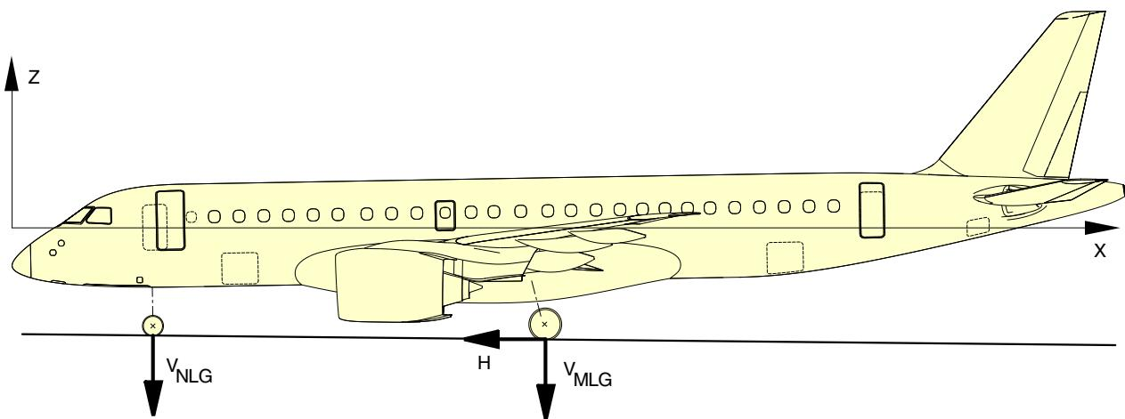
**NOTES:** STEADY BRAKING:  $H = 0.30 \cdot V_{MLG}$
