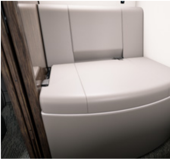
Externally serviced odorless vacuum lavatory.
